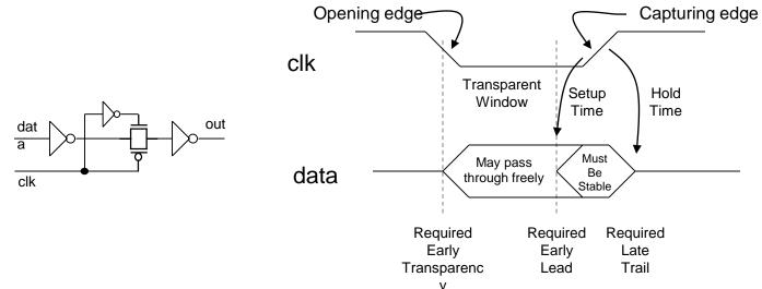
Inputs may switch anytime in this window, so long as they are valid before the capturing edge of the clock, and remain valid until the hold time (+ skew)
