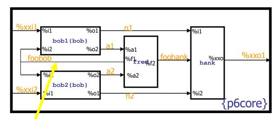
The nodes in p6 core have RCDLY and need to be timed, but before we can do that we need to extract the Rs and Cs. This occurs during the FC RCEXT. One output format for FC RCEXT is a NTCL file:
